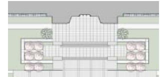
NEW NORTH ENTRY STEPS AND SYMMETRICAL RAMPS
