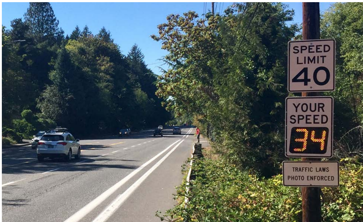
Figure 3. Speed reader board assembly, SE Beaverton-Hillsdale Highway, City of Portland
