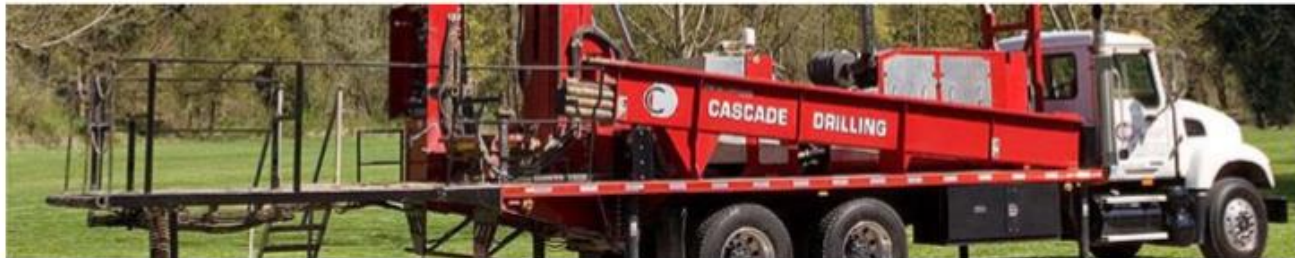
Sonic Drill Rig (For Exploration South of Capitol)
