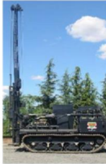
Track-Mounted Mud-Rotary Drill Rig
